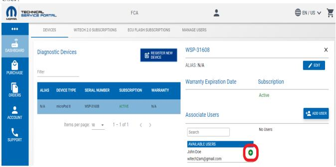
Now the VCI device has a subscription and users assigned to it and is ready for use with wiTECH 2.0.
