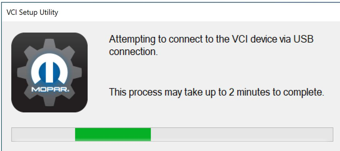
If you receive an error message stating that the device could not connect, ensure that the VCI is connected correctly to your computer with the USB cable, and click **Refresh** to try again.
