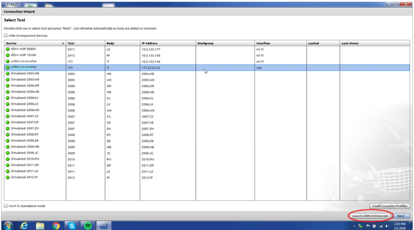
4. Click the “Launch DRB III Enhanced” button and accept the EULA that is presented. A warning will be presented indicating that Enhanced DRB III Emulator is not installed. Press “OK” to start the installation process.
