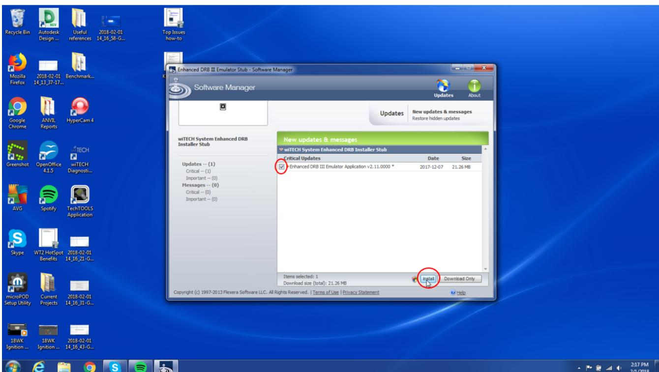
7. Follow through any dialog prompts to complete installation. Once installation has completed, open the wiTECH Diagnostic Application and select the microPOD II device using the Connection Wizard. Click the “Launch DRB III Enhanced” to open the Enhanced DRB III Emulator. The emulator will appear as shown below if you are connected to a vehicle.
