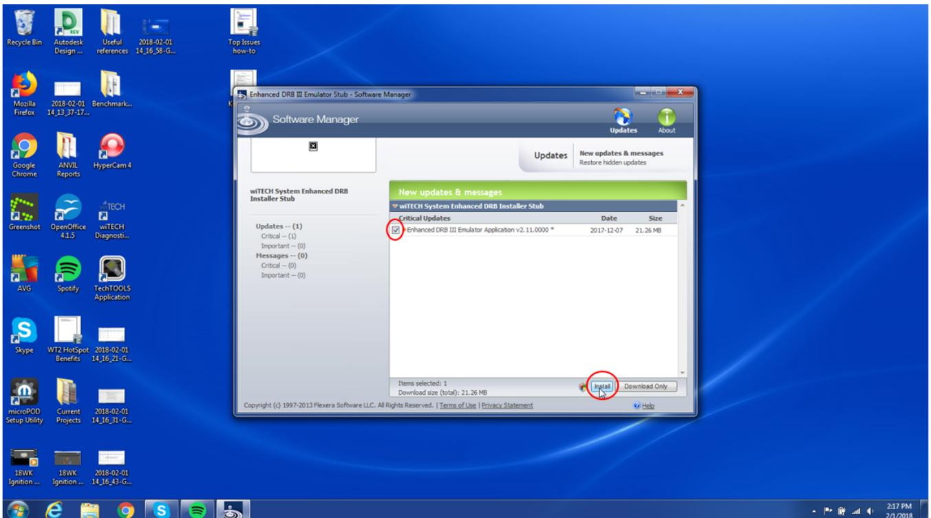
7. Follow through any dialog prompts to complete installation. Once installation has completed, open the wiTECH Diagnostic Application and select the microPOD II device using the Connection Wizard. Click the “Launch DRB III Enhanced” to open the Enhanced DRB III Emulator. The emulator will appear as shown below if you are connected to a vehicle.
