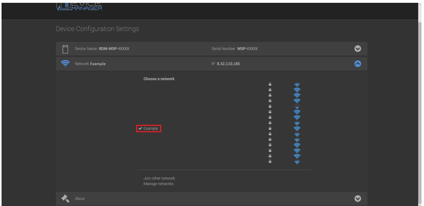
14. The VCI device is now connected to Wi-Fi. Close the Device Configuration Settings tab and the VCI Setup Utility.
